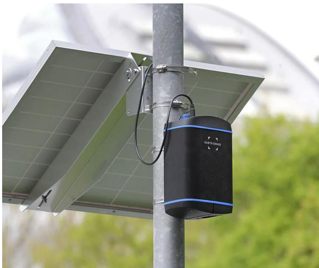
Figure 3-1 Typical Earthsense Zephyr Monitor
